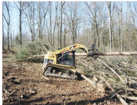
Low ground pressure tracked skid steer used on frozen ground to minimize ecological footprint
